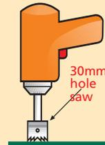
Drill a hole in the place that you have selected on the tank's top surface using a 30mm hole-saw.
