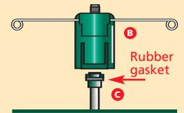
Fit the transmitter (B) onto the top of the tube and push it down firmly. Use the correct type of screws depending on whether the tank is steel or plastic to tighten the transmitter down fully onto the tube.
